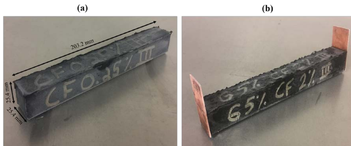
Figure 5.2 Preparation of prismatic asphalt mastic specimens: (a) demolded asphalt mastic specimen, and (b) asphalt mastic specimen with attached copper electrodes.
